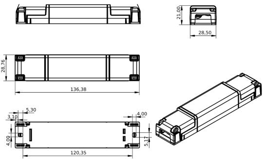
Figure 9: Mechanical dimensions
