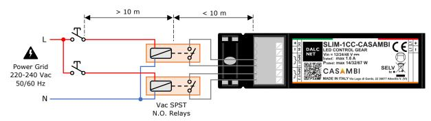
Figure 4: Local Command connection diagram for Long Distances
