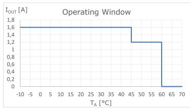
Figure 7: Operating Temperature Window
