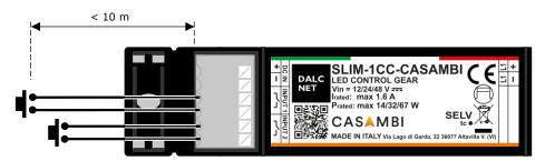
Figure 3: Local Command connection diagram for Short Distances
